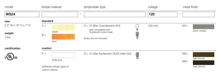
material details mounting details shade project: the standard shade material is 2-ply wood veneer with a poly core lamination and surface coating. The material is cleanable with soap water and cloth or household spray cleaners. type: the custom white poly material can also be made in other colors. crossbar with ground screw quantity: hardware octagonal junction box in wall, all hardware is steel or aluminum with a powder coat finish. 3.5" hole spacing notes: canopy slides up stem for mounting
